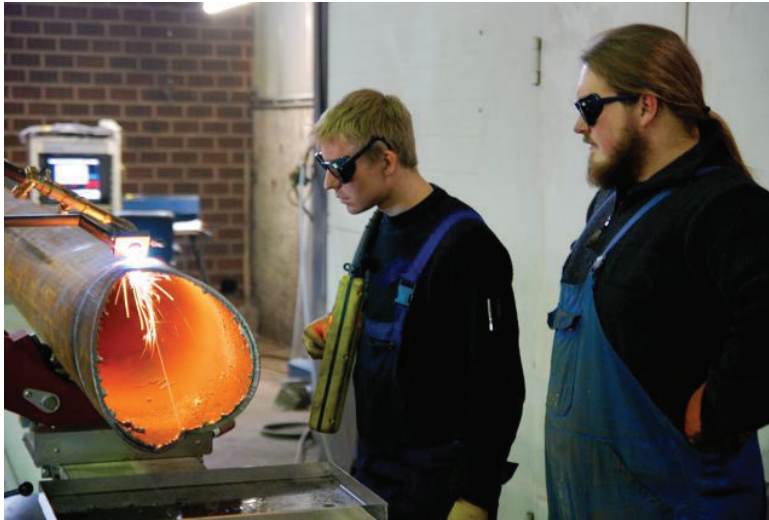
◀ Figure 13 (left). CNC plasma cutting of steel pipes.
