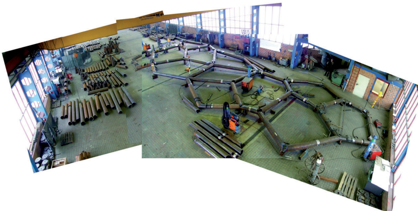
◀ Figure 15. Test assembly of tree structure mesh.
