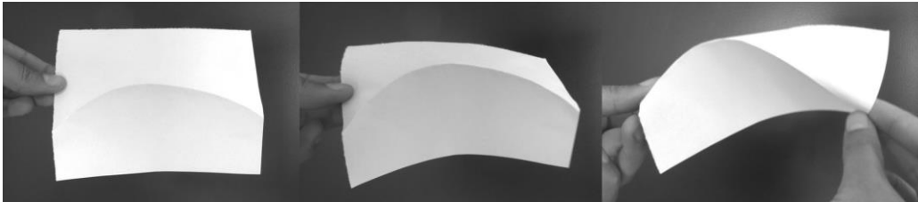
Figure 3: The picture on the left shows the initial state of the curved-crease pattern. The picture in the middle shows the basic shape generated by folding around the curved crease. The picture on the right shows a twisted variation of the basic shape obtained through physical interaction with the paper model.
