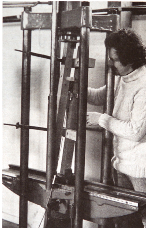
Fig 5. Testing for shear stiffness.
