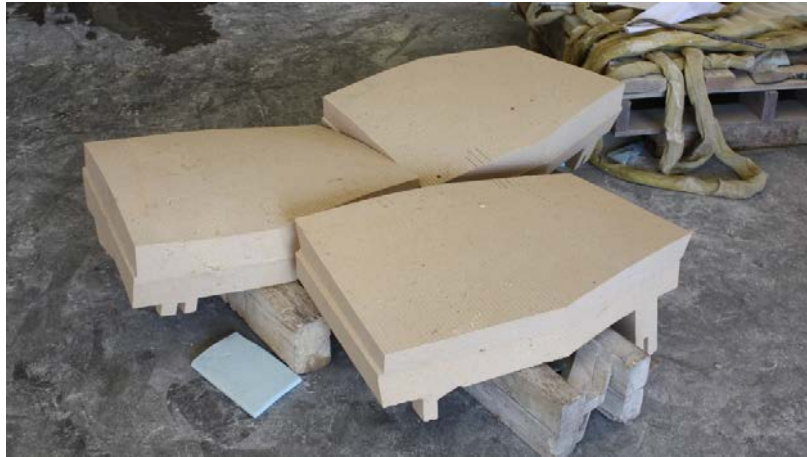
Figure A.21: Stone blocks that have been fabricated using digital fabrication methods [19]
