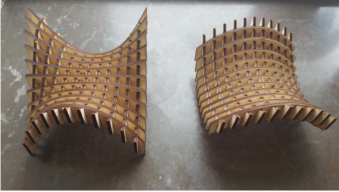
Figure 2.8: Two examples of surfaces made of ribbed wood structures. To the left is a "Monkey saddle"- surface described in Cartesian coordinates z = x^3 - 3xy^2 , to the right a Hyperbolic paraboloid z = (y^2)/(b^2) - (x^2)/(a^2)
