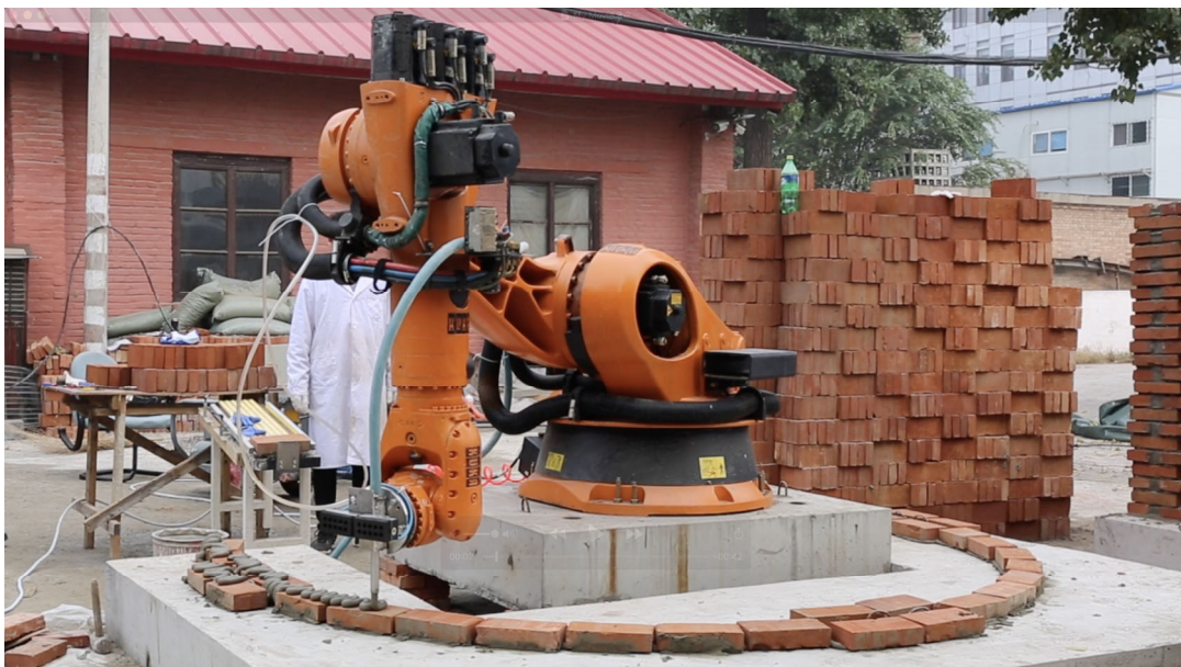
Figure 8 Lab Testing of the Planned Path and the Automatic Brick Assembly System.
