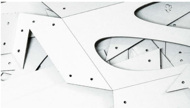
Figure 11: Gridshell components are tagged and cut with a Digital Cutting Plotter
