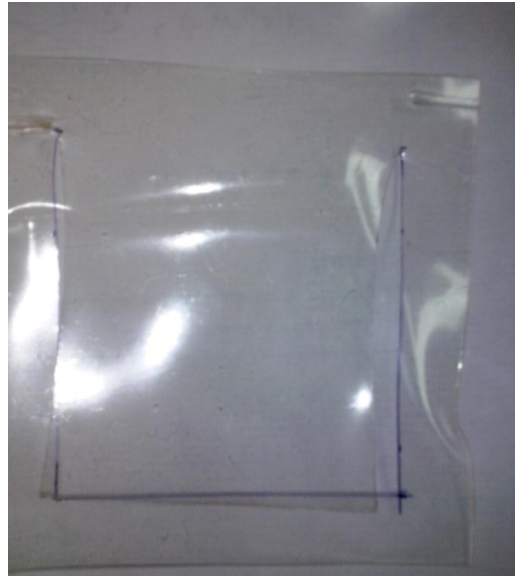
Fig. 100 Photos of the 0.7mm SMP sheets after exposure to air flow heated up to 40 degrees Celsius.
