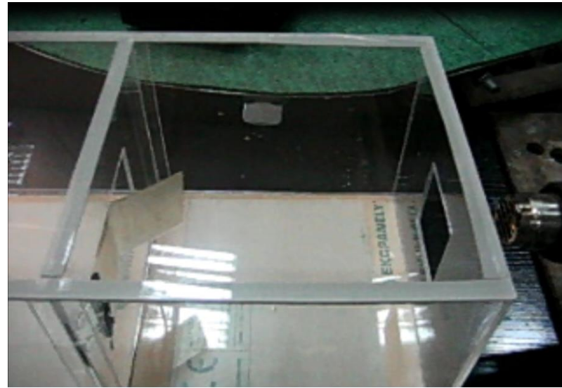
Fig. 108 Pictures taken for the last 2mm SMP sheet placed in the internal window within the model and exposed to hot air heated up to 37 degrees celsius, and the pictures show the movement of the sheet from 180 degree to 45 degree to 90 degree, allowing the air to flow in the model.
