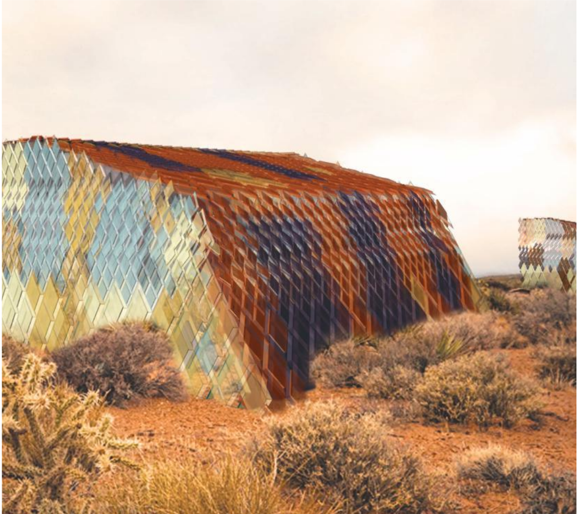
Fig. 89 The artist studio fixes itself directly on the desert floor, much like the lizard. The individual panels gleam in the sunlight while collecting heat and energy. The structure maintains a slight tilt in the roof and south façade in order to be optimally positioned to the sun angle. ( Ibid )
