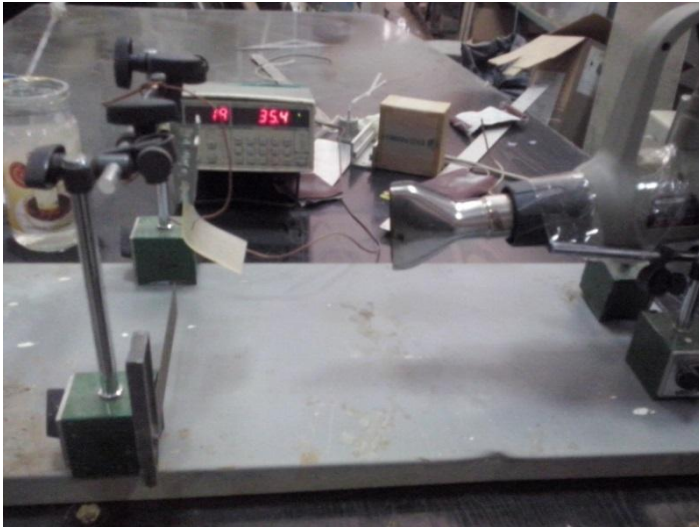
Fig. 103 Pictures taken for the 2mm thick SMP sheet after bending it by hand then exposing it to hot air heated up 35 degrees Celsius which made it retain its original flat shape again.
